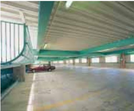
A temporary propped Hi-Bond composite decking system was used with a 120mm concrete topping. The seismic resisting system consists of eccentrically braced frames (EBF's) on major elevations and six moment resisting frames at 10.4m centres, across the building. All columns were concrete encased as the floors were constructed.
