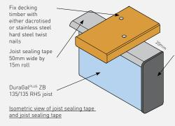
Seal top and sides of end cap to joist or bearer with a bead of a neutral, flexible paintable sealant. Bottom not sealed to allow moisture to drain.
