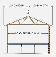
DuraGal<sup>PLUS</sup> Adjustable Piers can also be used around the perimeter of brick veneer houses. This makes it possible to erect the floor, frame and roof prior to the bricklayer coming to site.
