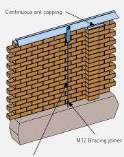
Threaded rod anchored into concrete to engineer's specifications
