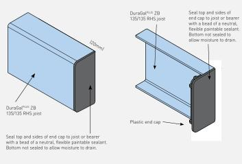
Isometric view of joist with end cap sealing PART Isometric view of joist with end cap sealing
