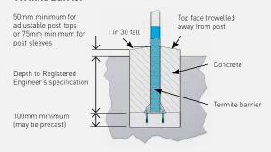
The termite barrier shown is only required for through columns with fixed post top components. Refer to AS 3660.1 for details.
