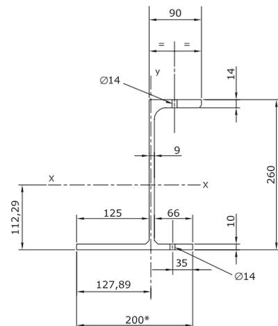
\*Platform leg available in 300mm width. (Section details and load tables available on request)
